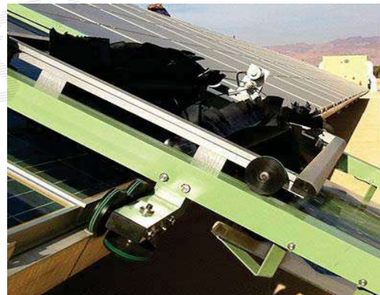
Fixed installed brush (dry) cleaning system
