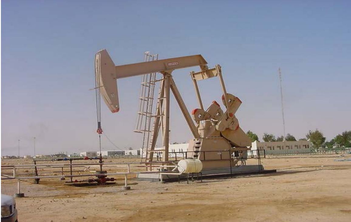
Typical Oil Well – With Pump-Jack (Khalda)
