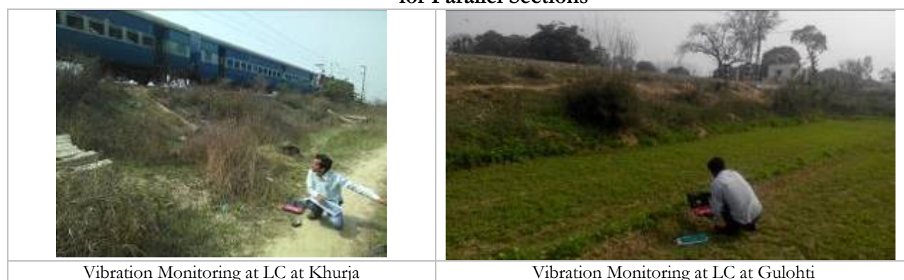
Figure 5.12: Photographs of Vibration Level Monitoring along the Existing IR Track for Parallel Sections
