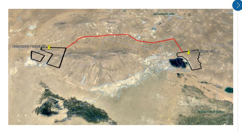
The project also includes the development of an Overhead Transmission Line (OHTL) with a rating of 500kV single circuit. This OHTL will be shared between ACWA Power's Dzhankeldy 500MW Wind Farm and the ACWA Power Bash 500MW Wind Farm. The alignment of the Dzhankeldy-Bash 128.5 km OHTL is approved by JSC National Electric Networks of Uzbekistan and will connect to an existing substation in Karakul.
