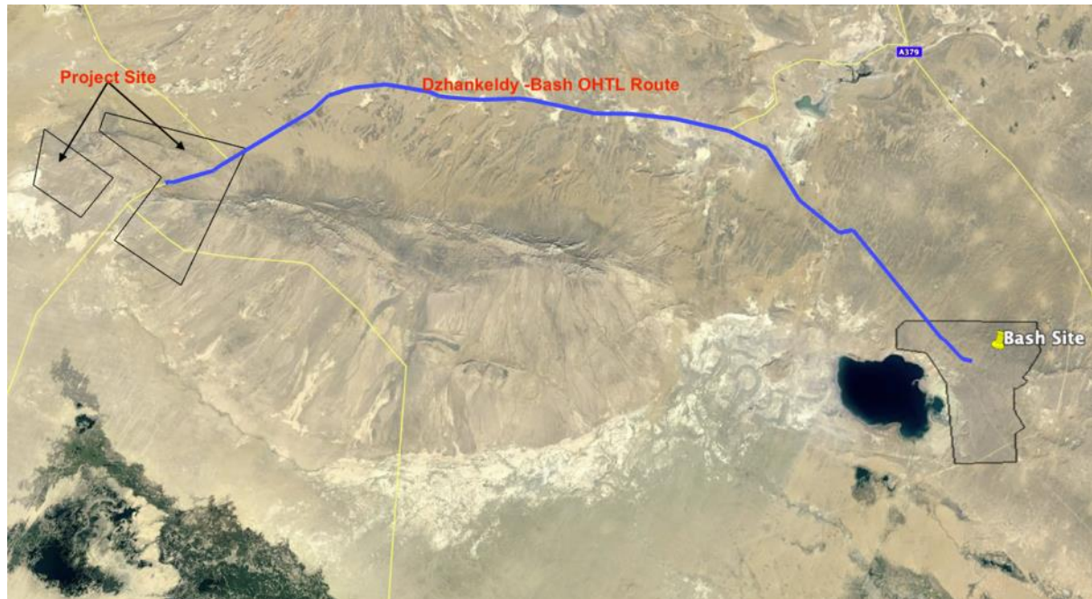
Figure 2-3 Alignment of 128.5km OHTL from the Dzhankeldy Wind Farm to Bash Site
