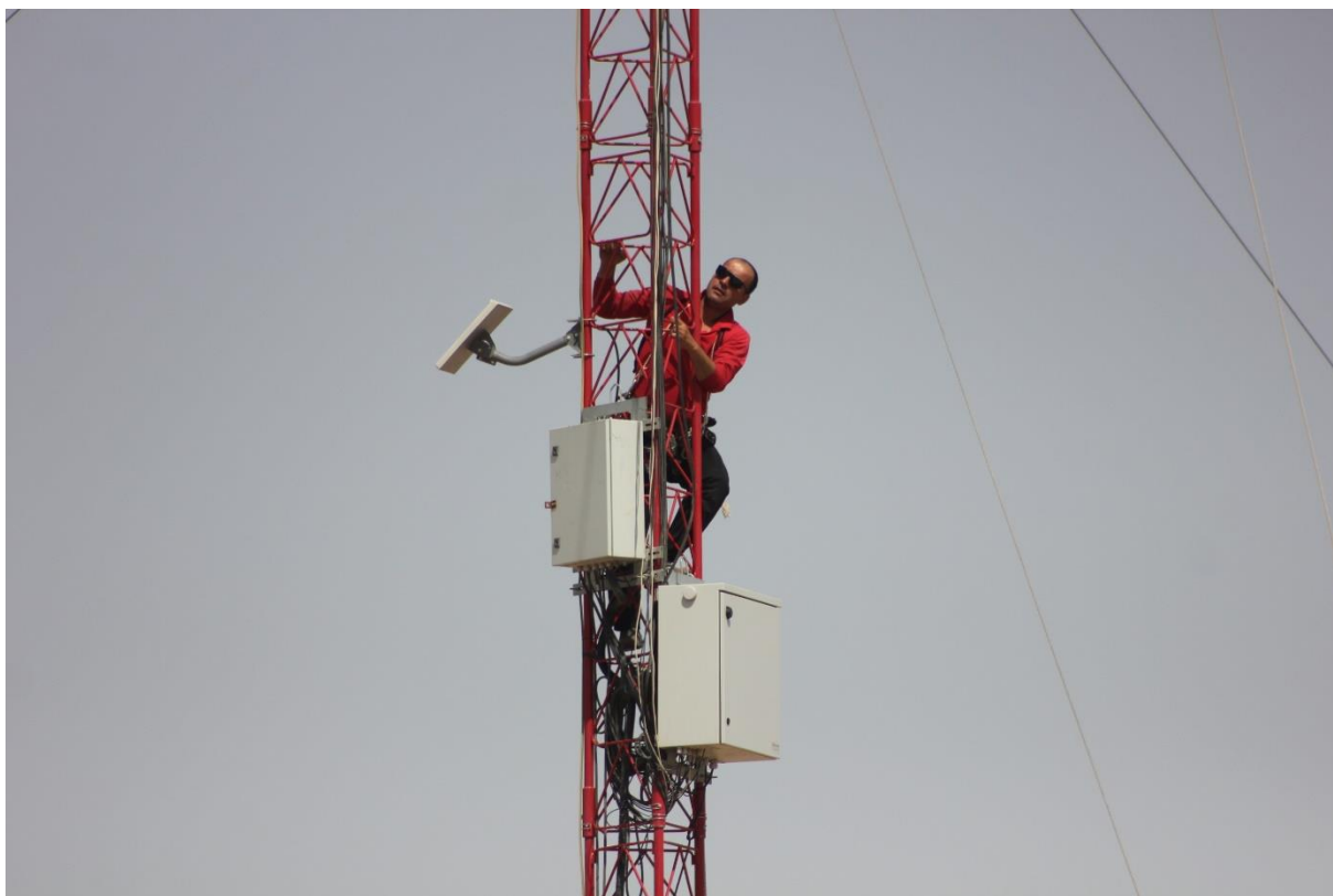
Bat detector collection from weather mast in Dzhankeldy project area
