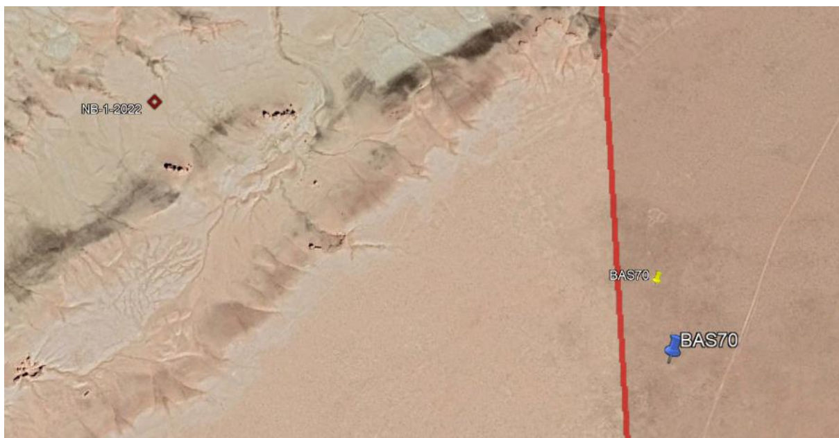
Figure 7-12 Microsited turbine BAS70 (Blue marker) beyond 750m buffer of Golden Eagle Nest
