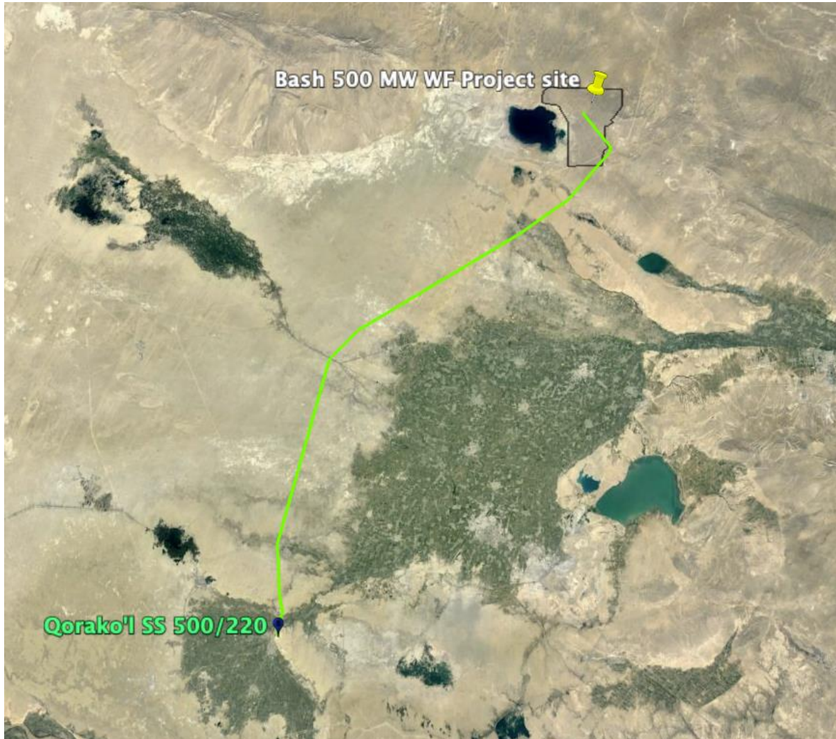
Figure 2-16 Location of 162 km OHTL Route from the Project Site to Kurakul Substation
