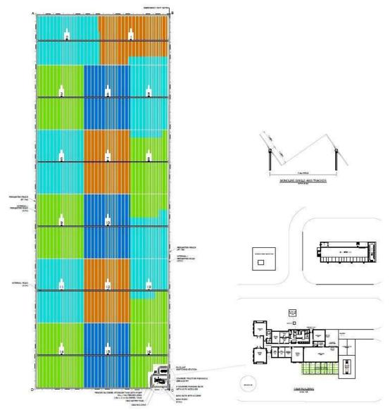
Figure 3-4: Buildings' location within the project area (location might change due to final 22 kV grid connection design; different color of modules indicates sections being connected to different inverters)
