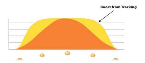
Figure (6-2): Daily power production, fixed tilt versus tracking Source: First Solar
