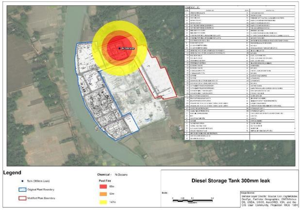
Figure 5.6 Threat Zone Plot –300 mm leak (Worst Case)
