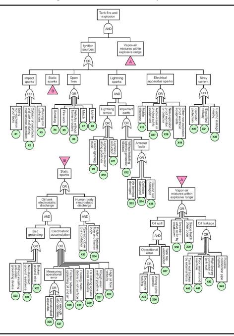
Figure 5.2 Event Tree Analysis - Tank Failure
