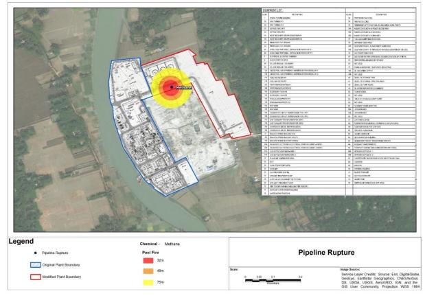
Figure 5.10 Threat Zone Plot – Temporary Gas Pipeline Rupture
