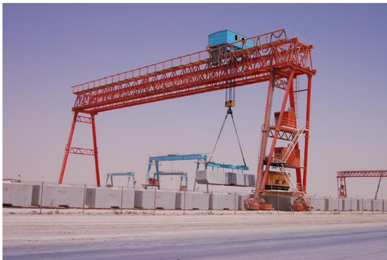
Figure 3-13: Example of Precast Concrete Blocks Stored in Yard (Source: http://www.npp.com.qa )
