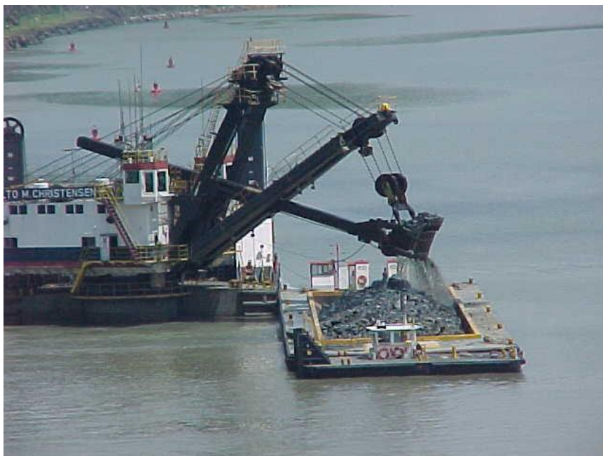
Figure 5-7: Example of a Dipper Dredger (Source: www.czbrats.com )
