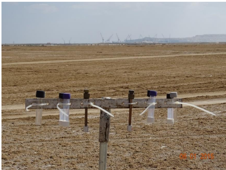
Figure 6-31: Close-up of the Diffusion Tubes on the Stand (Photograph taken on 6-Jan-2015)
