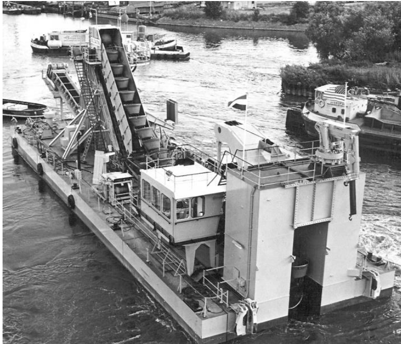
Figure 5-8: Example of a Bucket Chain Dredger (Source: http://www.dredging.org/ )
