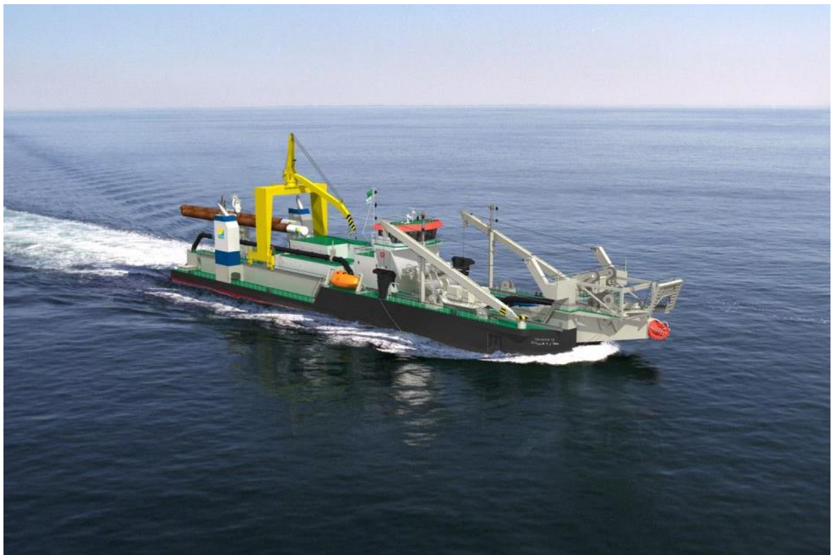
Figure 3-8: Photograph of a Typical Cutter Suction Dredger (Source: http://www.dredgingtoday.com/ )
