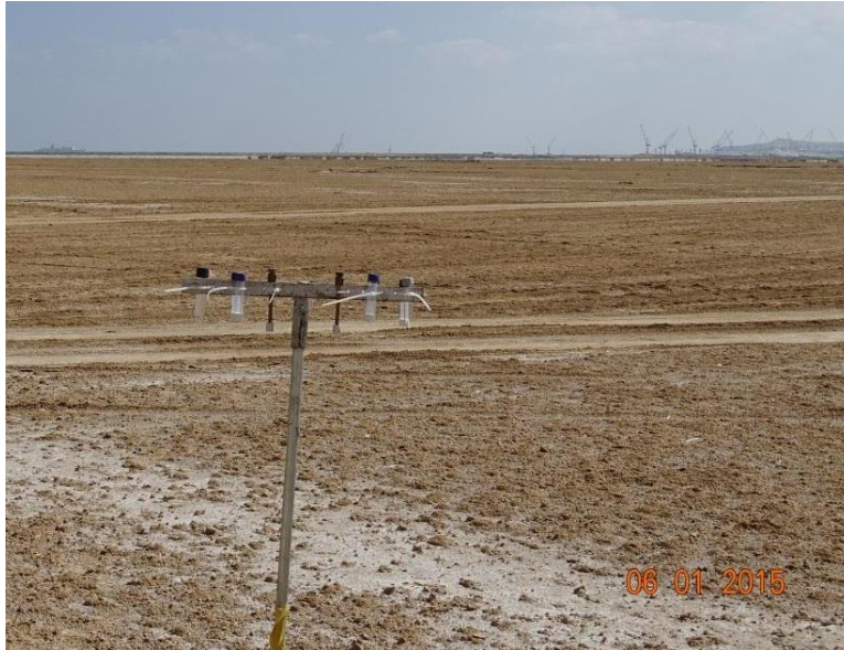
Figure 6-30: Diffusion Tubes Mounted on Stand (Photograph taken on 6-Jan-2015)
