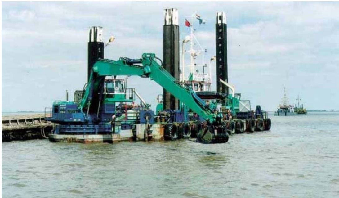
Figure 5-5: Example of Back Hoe Dredger (Source: http://www.dredging.org/ )
