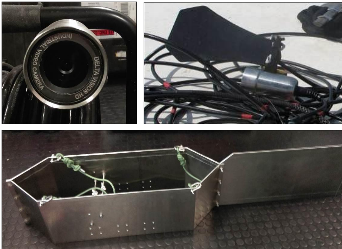
Plate 3-3 Delta Vision HD camera and towfish frame
