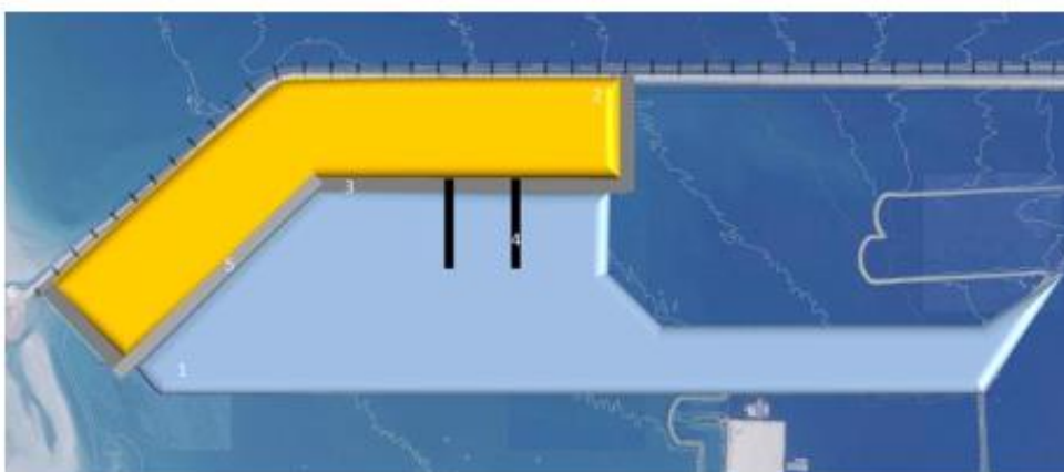
Figure 1.2: Schematization of the Works (1 to 5 indicate dredging, reclamation, revetment, jetties and quaywall, respectively)
