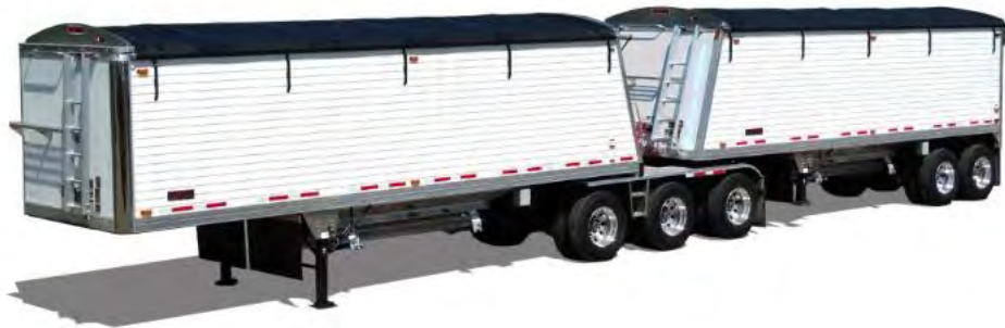
Figure No. 7.18. Specialized vehicles for bulk transport, high speed unloading hopper and coupled tandem.
