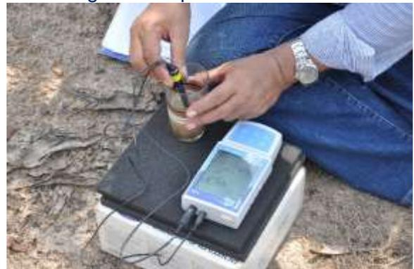
Testing soil Electrical conductivity (Ec)
