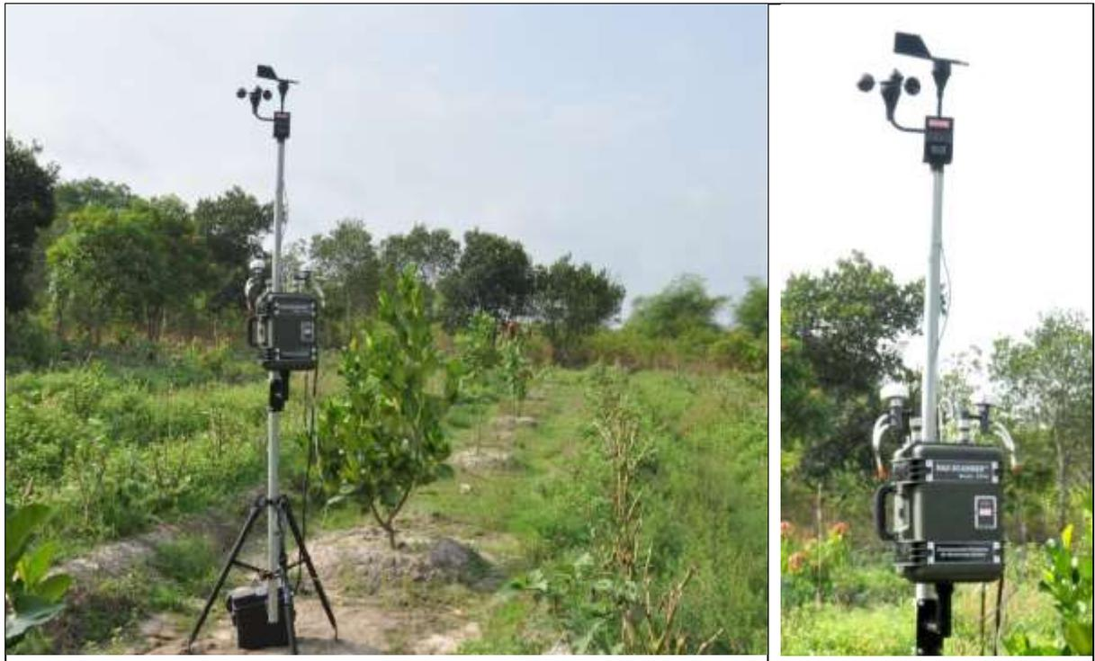
Figure 7-2: Air Quality Measurement Device
