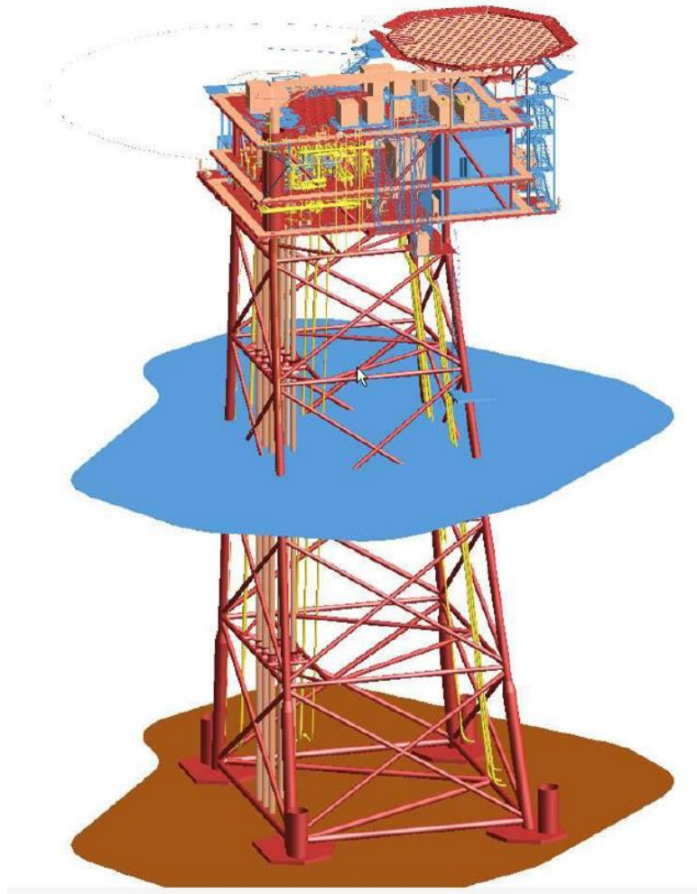
Figure 3.0-2: Simulation of the York platform in the North Sea
